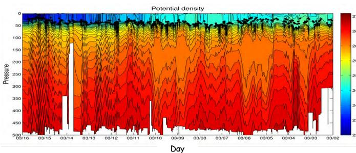
**Figure:** uCTD potential density field (color) and the black dots are the mixed layer depth, defined by the potential temperature threshold of 0.2°C. When the wind is more intense, mixed layer should be deeper.
