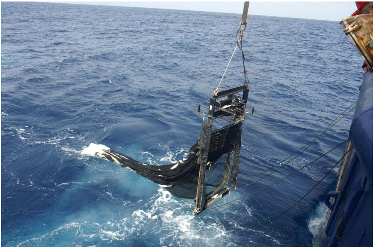
The MOCNESS net is being deployed from the stern of the METEOR. Photo T. Tanhua.
